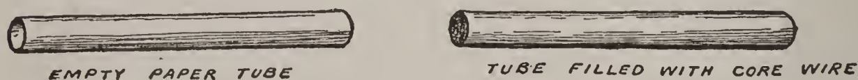
FIG. 158. — Empty Paper Tube, and Tube filled with Core Wire preparatory to winding on the Primary.
