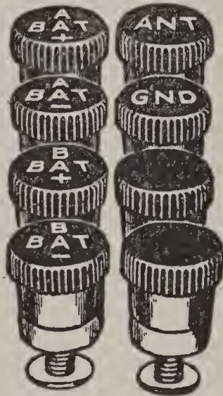
FIG. 226. — A Set of Marked Binding Posts.
