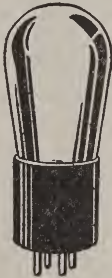
FIG. 225. — A Type "300 A" Detector Tube.
