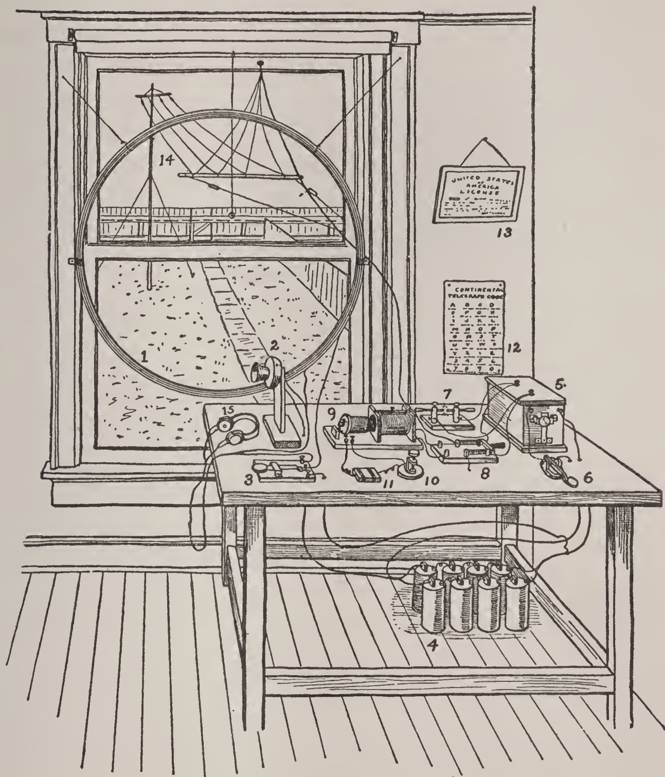
FIG. 246. — A Complete Wireless Telephone and Telegraph Station for Amateurs. 1. The Telephone Coil. 2. The Telephone Transmitter. 3. Double-Contact Strap-Key. 4. The Battery. 5. Spark Coil. 6. Key. 7. Spark-Gap. 8. Aerial Switch. 9. Loose Coupler. 10. Detector. 11. Fixed Condenser. 12. Code Chart. 13. Amateur License. 14. Aerial. 15. Telephone Receivers.
